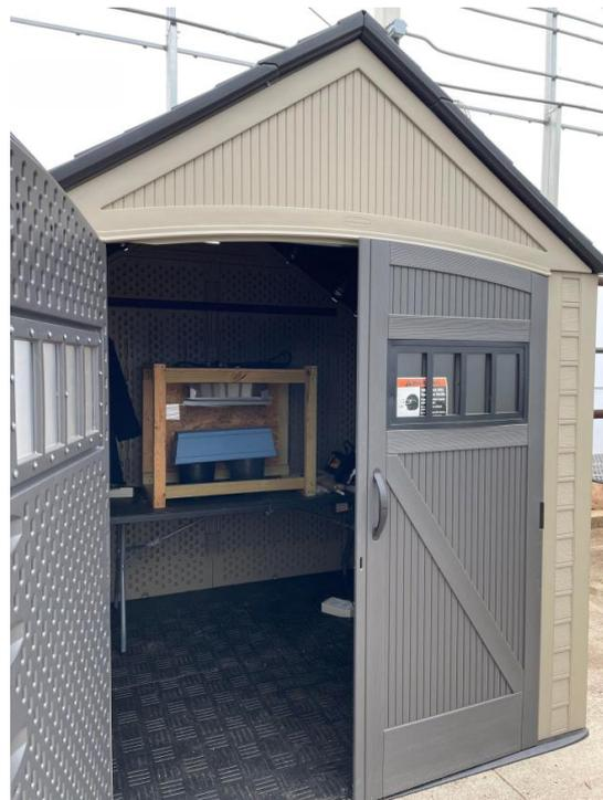
**Figure 1.** Custom-built UV light chamber used for UV-B and UV-C application on the lettuce seedlings in the current study. UV-B and UV-C lamps were installed on the top panel of the wooden structure, and the outer door remained closed during operation.
