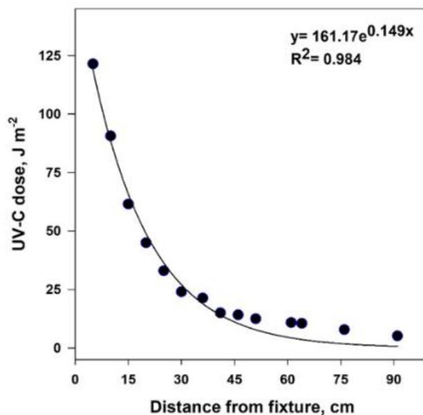
**Figure 2.** Nonlinear model adjusted to represent UV-C light intensity as a function of distances between the source of light and the targets. The determination coefficient ( $R^2$ ) of the fitted model is also shown.
