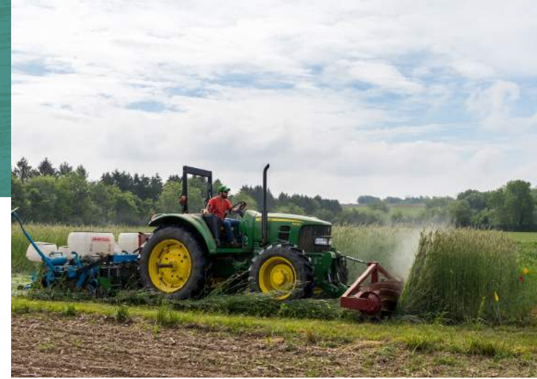
The front-mounted roller crimps a cover crop such as cereal rye to form a thick mulch into which a cash crop such as soybeans can be simultaneously planted. The mulch effectively suppresses weeds.
