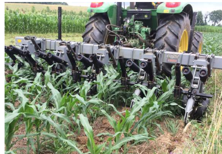
An innovative tractor-mounted high residue cultivator is utilized to manage weeds as a last resort when complete weed control by rolled cover crop is not achieved.
