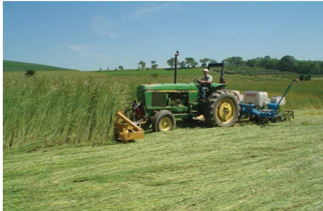
Rodale Institute's Jeff Moyer uses a front-mounted roller-crimper and a rear-mounted no-till seeder to simultaneously terminate the winter rye and hairy vetch cover crop and direct seed soybeans.
